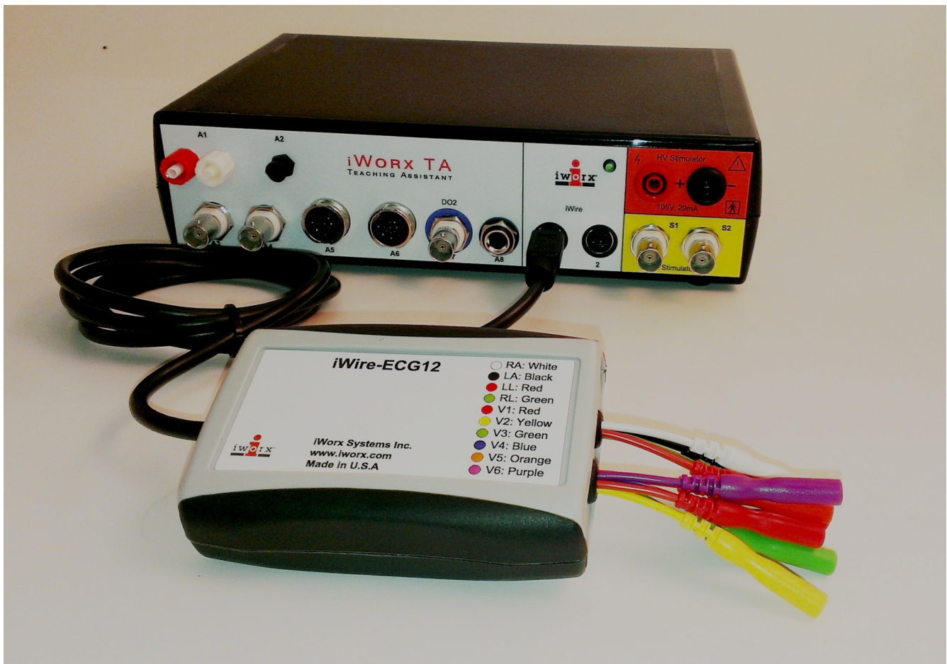
Figure HH-13-S3: iWire-ECG12 connected to the iWire 1 port of the IXTA.
